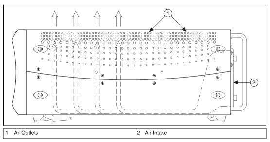
Figure 2-1. PXI-1052 Chassis Airflow Side View
